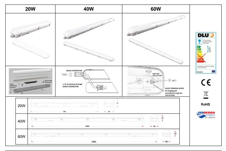
Fixed IP65 wall-mounting fixture, integrating an array of high power LEDs geared by a constant current LED driver. IP65 QUICK CONNECTOR at the L,N,G entrance. The other end is closed, but with a precut hole to eventually receive an IP65 CLAMPING CABLE GLAND given in the accessory bag: at its correspondence inside the fixture, a QUICK TERMINAL BLOCK is internally wired with L,N,G ready for the eventual looping to a subsequent fixture.
